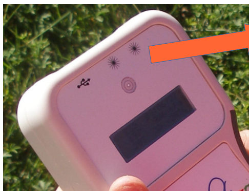
The Sun spot is on the center of the target : the photometer is pointed.
