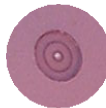
The Sun spot is on the center of the target : the photometer is pointed.
